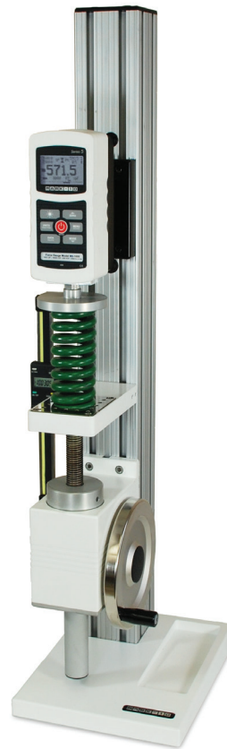
The TSF is shown testing a compression spring, with a Series 5 digital force gauge and digital travel display
